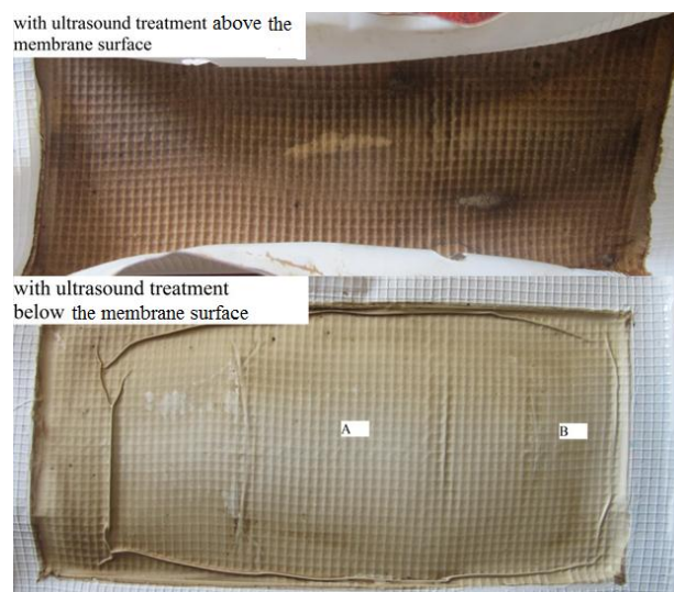
Fig 6. Image of the membrane surface after membrane clarification of pomegranate juice with ultrasonic treatment
