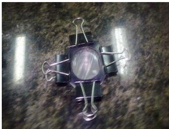
Fig 1. WVP test for a film sample
