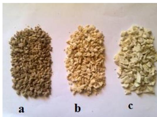
**Fig 1.** WS/LDPE biocomposite granules contain raw WS (a), BWS (b), and BWS pulp (c)
