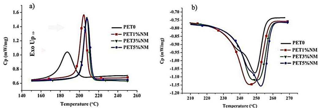
Fig 3. DSC curves of neat PET and its nanocomposites, cooling (a) and heating (b) processes
