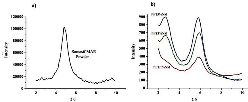
Fig. 1. WAXD analysis of mica powder (a) and PET/mica nanocomposites
