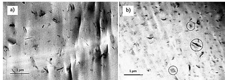
Fig. 2. TEM micrographs of PET nanocomposites containing 1 wt% (a) and 3 wt% (b) nano micas
