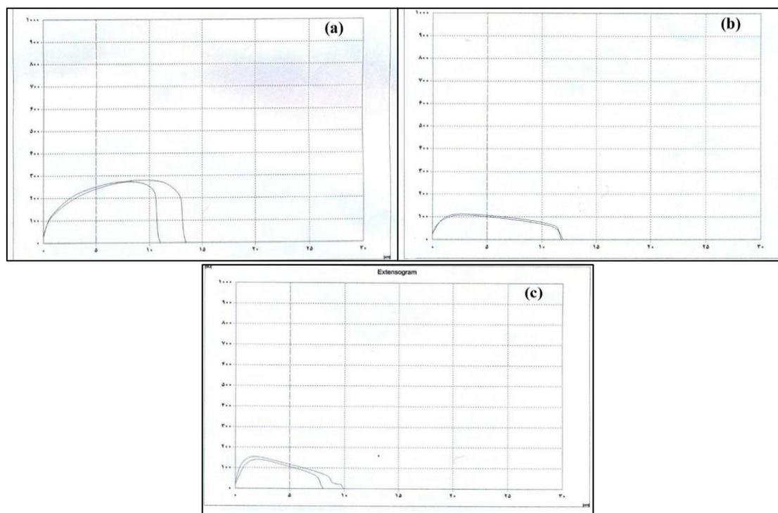
Fig. 2. Extensogram of flour with 64% (a), 82% (b) and 90% (c) extraction rate
