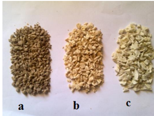
Fig. 1. WS/LDPE biocomposite granules contain raw WS (a), BWS (b), and BWS pulp (c) (Ansari, 2012).
