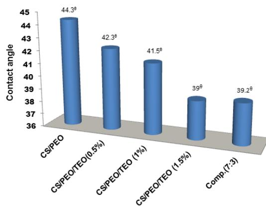
Fig. 10. Water contact angle for CS/PEO, CS/PEO/TEO nanofibers at different concentrations and polymer coated nanofibers with comp.(7:3).
