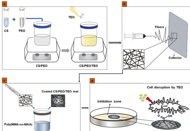
Scheme. 1. Schematic illustration of the procedure including a) preparation of CS/PEO and CS/PEO/TEO solutions, b) electrospinning of the polymer solutions to fabricate nanofibers, c) dip-coating by immersing CS/PEO/TEO electrospun mat into the poly(MMA-co-MAA) solution, d) assessment of antimicrobial activity by determination of inhibition zone for coated electrospun mats.
