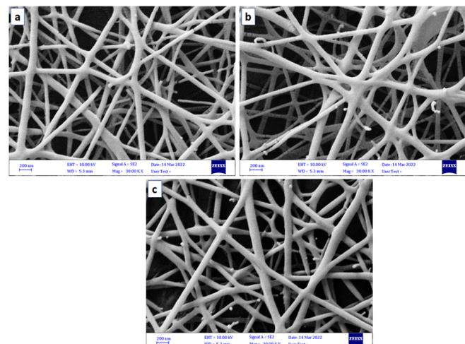
Fig. 5. CS/PEO/TEO nanofibers at concentrations of a) 0.5, b) 1 and c) 1.5% of essential oil.
