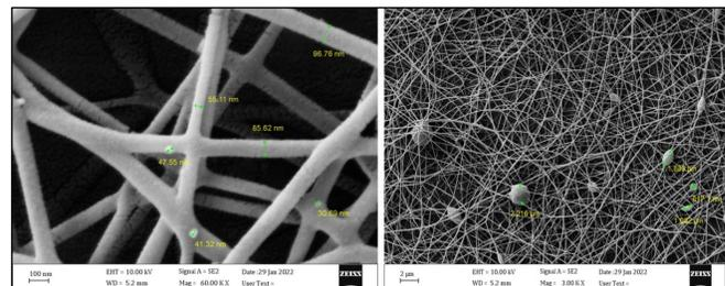
Fig. 4. SEM images of CS/PEO electrospun mat at the ratio of 50/50.
