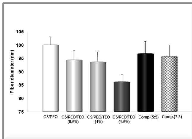
Fig. 7. Fiber Diameter for CS/PEO and CS/PEO/TEO electrospun mats (coated and uncoated).
