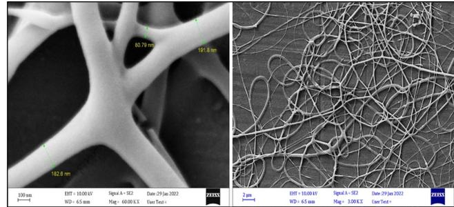
Fig. 2. SEM images of CS/PEO electrospun mat at the ratio of 20/80.
