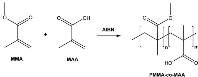
Fig. 1. Chemical structure of poly(MMA-co-MAA).
