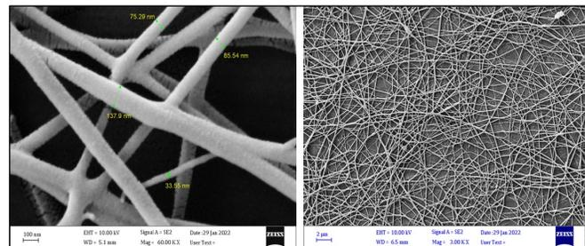
Fig. 3. SEM images of CS/PEO electrospun mat at the ratio of 40/60.
