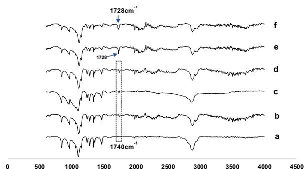
Fig. 8. FTIR spectra recorded for a) CS/PEO, b) CS/PEO/TEO (0.5%), c) CS/PEO/TEO (1%), d) CS/PEO/TEO (1.5%) and %, e and f) coated nanofibers with poly (MMA-co-MAA); comp.(7:3) and comp.(5:5) respectively.
