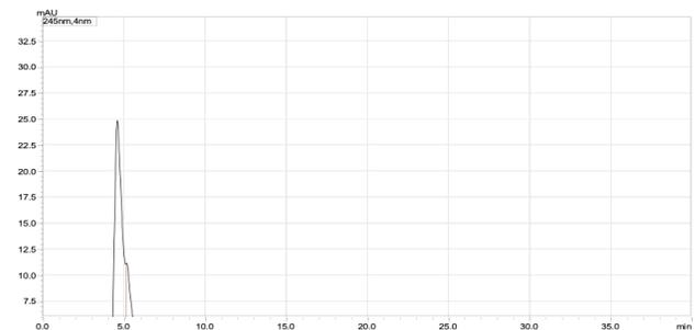
Fig. 13. L-Ascorbic acid in Fard Date Powder at 245 nm.
