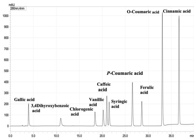
Fig. 3. Chromatogram of Phenolic Acid Standards Detected at 280 nm.
